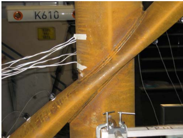
Figure 10. X45-1C chord plastification failure as the chord flattens at the joint; typical failure for type 1 joints.
