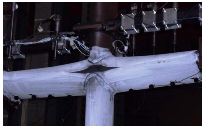
Figure 7. X90-2T failure mode showing an example of chord tearing for a tension test.
