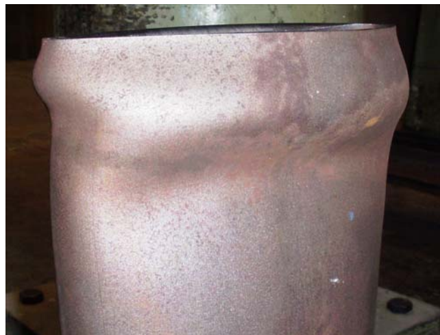
Figure 5. Local buckling of EHS cross-section from stub-column test.
